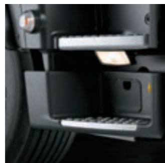
Manoeuvring light in co-driver's entry lights up the visible area of the ramp mirror.
