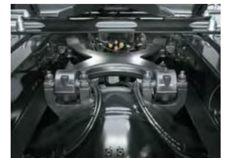
Weight-optimised X control arm with stabiliser and control arm function for semitrailer tractors and high-load roll stabilisation for 6x2 vehicles.
