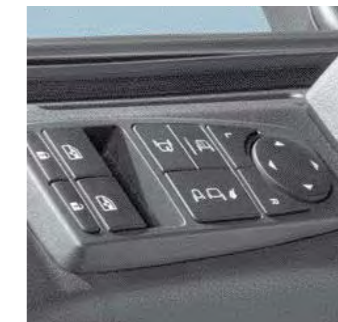
Ergonomically styled door control module for locking, mirror adjustment and window lifters.
